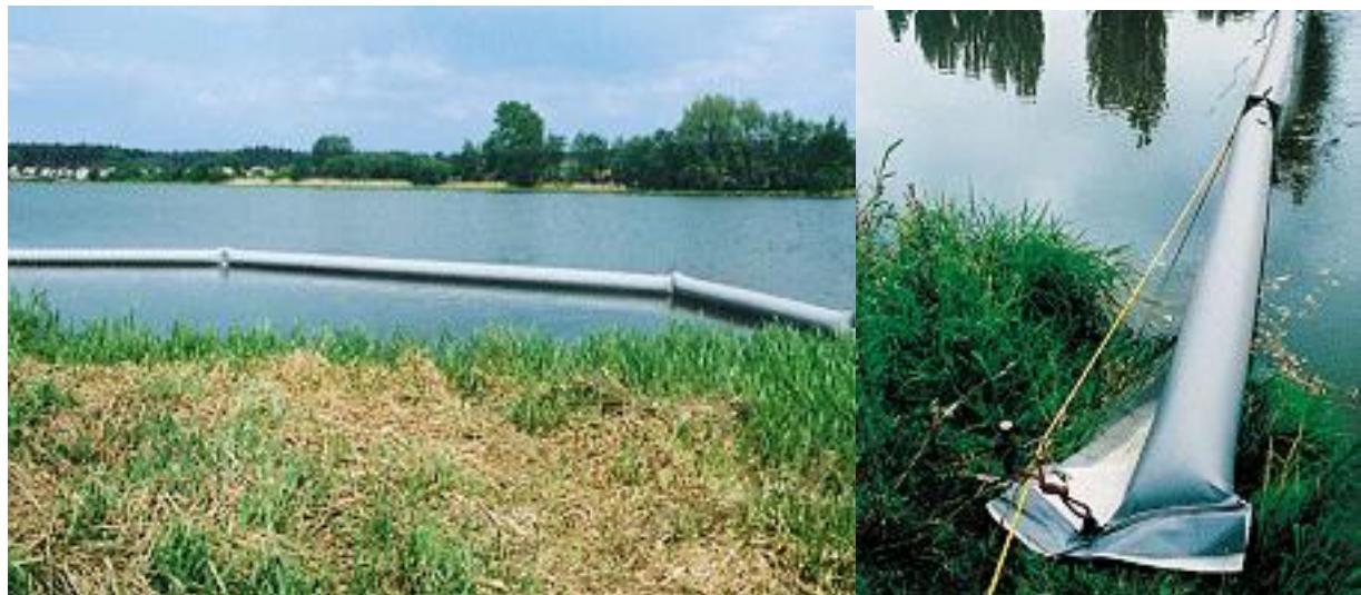
**Fig 2** The cylinder-shape barrier (Photo autor)
