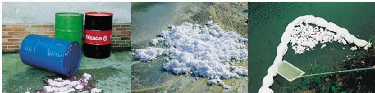
**Fig 8** Examples Hydrophobic absorptive loose absorbent (no woven textile)
